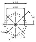
All corners must be deburred! According to ISO 2768-m
