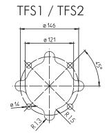
All corners must be deburred! According to ISO 2768-m
