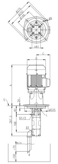
L = Leakage hole S = Mounting plate, please refer to the cut-out of mounting hole
