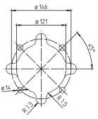
All corners must be deburred! According to ISO 2768-m
