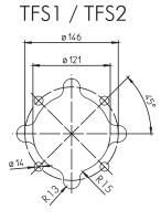
All corners must be deburred! According to ISO 2768-m
